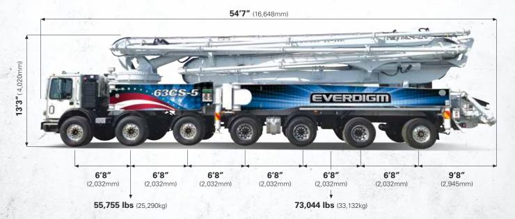
Based on Model MACK MRU 613 with 2116 pump cell. Dimensions will vary with different truck makes, models and specifications. Weights are approximate and include pump, boom, truck, driver and some fuel. Varies with options selected.
