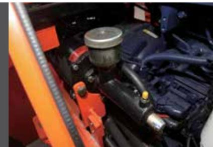
The booster pump delivers a higher augmented-thrust ratio, more stable braking performance, and more convenient daily maintenance thanks to its being mounted on the body's side.
