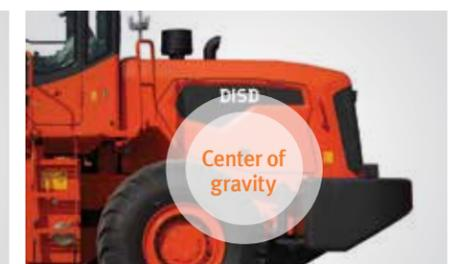
The whole center of gravity has been moved backward, and the real axle load bearing proportion has been increased to 54% resulting in a tipping load 10% higher than the industry level and greatly improved product stability.
