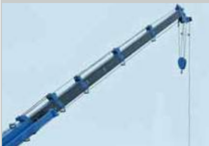
Patented Two Tele Boom Cylinders Mechanism (SS7506S)
