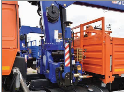
Rotator Type Front Outrigger
