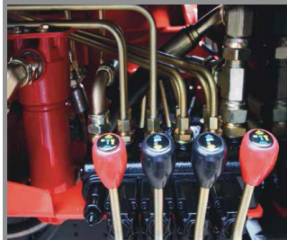
Enlarged Capacity for Outrigger Valve
